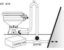
water in the bowl, the discharge hose should be looped upward about eight to ten inches above the base of the toilet and as near to the toilet as can be practically accomplished without creating an unsightly plumbing situation.
