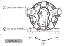
CAUTION: The pressure setting for full bypass must be at least 8psi higher than the shut-off pressure of the pump. If the switch and bypass is adjusted too closely, the bypass and switch shut-off can overlap and the pump will not shut off.
