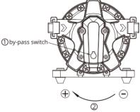
CAUTION: The pressure setting for full bypass must be at least 8psi higher than the shut-off pressure of the pump. If the switch and bypass is adjusted too closely, the bypass and switch shut-off can overlap and the pump will not shut off.
