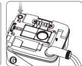
Press and hold the exhaust button and drain again
