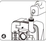
Lift the waste water tank and add 1-2L of clean water
